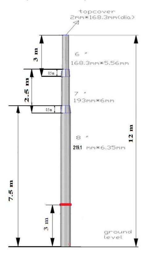
Drawing no.5 - Steel Tubular Specification 10 Meter.
