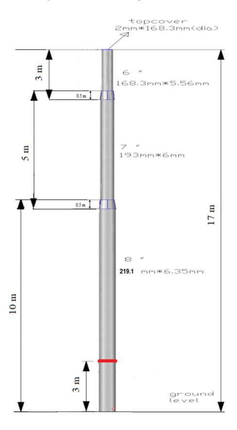
Drawing no.2 - Steel Tubular Specification 15 Meter.
