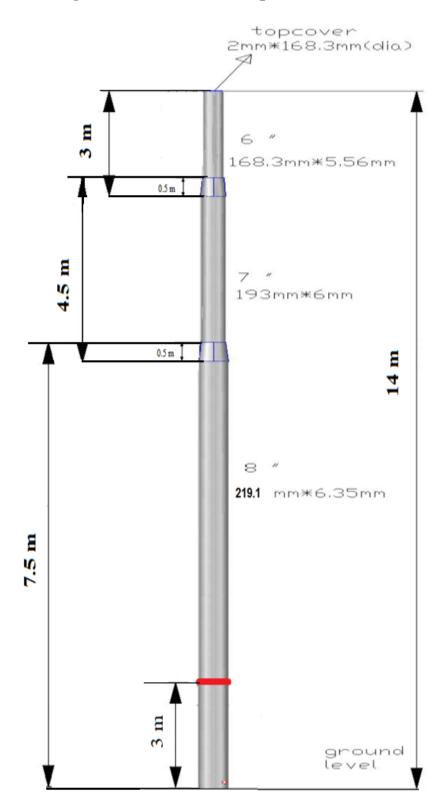
**Drawing no.4 - Steel Tubular Specification 12 Meter.**
